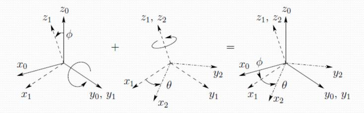
$$\begin{array}{rccccccc} p^0 &=& R_1^0 p^1 \\ p^1 &=& R_2^1 p^2 \\ p^0 &=& R_2^0 p^2 \\ p^0 &=& R_1^0 R_2^1 p^2 \end{array}$$
