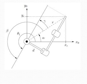
$\theta_{1} = \alpha + \beta$   $\alpha = \arctan 2(x_{c}, y_{c})$   $\beta = \gamma + \pi$   $\gamma = \arctan 2(\sqrt{r^{2} - d^{2}}, d)$
