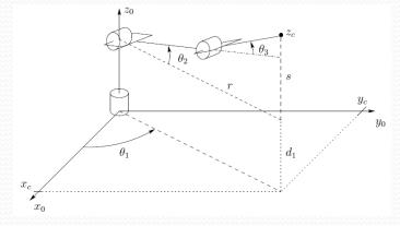
1. Projection onto link<sub>2</sub>-link<sub>3</sub> plan
